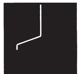
B-E paralleled by 680 \Omega
